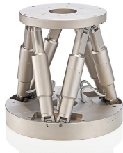
(a) CAD rendering of a Gough-Stewart platform, a general hexapod with 6 degrees of freedom and 6 actuators.
